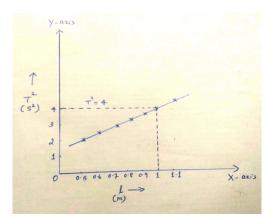
From  $(l, T^2)$  graph, length of the seconds pendulum = m
