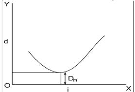
From the graph the angle of minimum deviation can be calculated.
